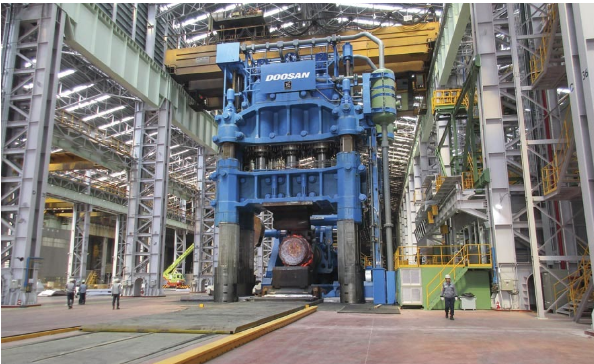
Figure 27 - 17,000 tonne forging press
