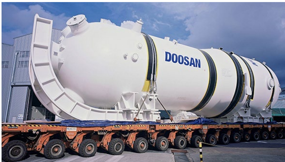
Figure 30 - Completed steam generators
