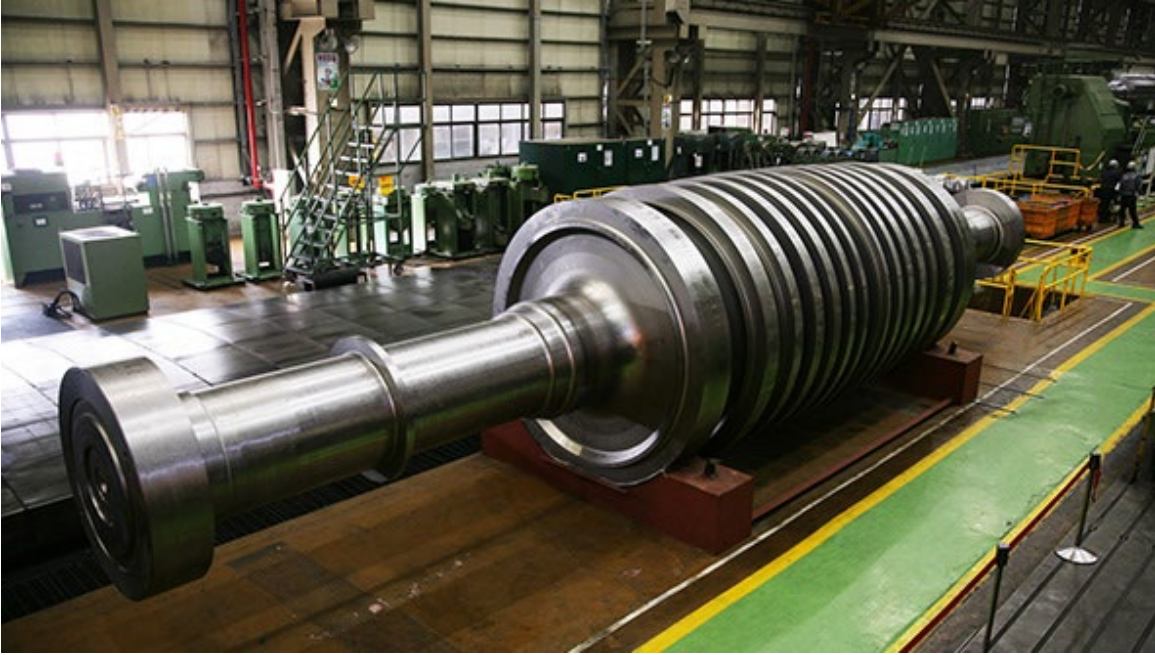
Figure 33 - Turbine Rotor shaft
